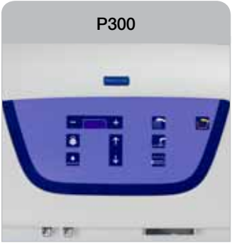
P300 The panel that offers the most advanced comfort and safety features: • Auto-fill+, three preset levels with possible afterfilling • Three-sensor scalding protection • Pre-programmed liquid dispensing system • Digital adjustment of water temperature • Digital adjustment of Hydrosound • Digital temperature display • Disinfectant container warning indicates when disinfectant is used up
